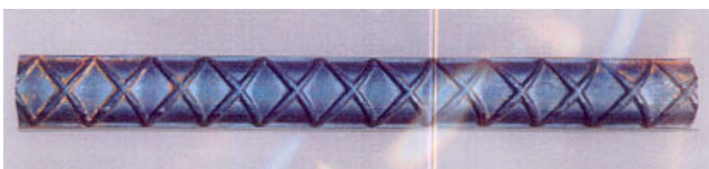
Front view of design of Steel Bar
